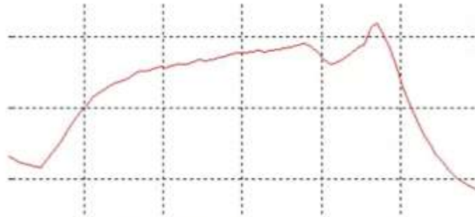
Figure 5 Room Temperature rise of 3.5F over 8 Hour Period
